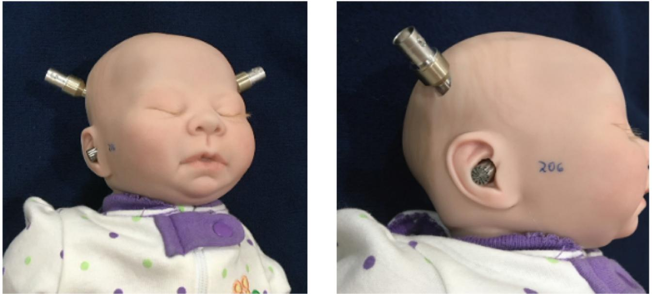
**Fig 2. Test mannequin showing microphone placement.** Holes were cut in the head of an infant mannequin, permitting the tip of each microphone to emerge from the molded auditory canal. The number written on the cheek of the mannequin indicates the calibration number of that microphone.
