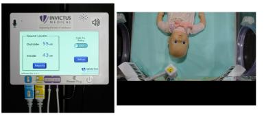
(1) The amount of attenuation produced by the ANC device was compared to the attenuation achieved by adhesive-affixed earmuffs (MiniMuffs, Natus Medical) in response to 11 alarm and voice sound sequences. The sequences were generated by different priority alarms from a patient monitor, an infusion pump, and a ventilator, either alone or in combinations. In a worst case scenario, alarms from all three were combined.
